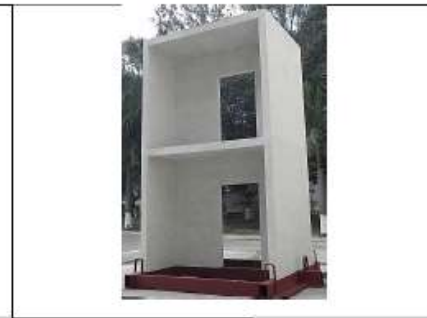
Fig. 3 Spraying and pouring of concrete over the EPS core skeleton and finished building model
