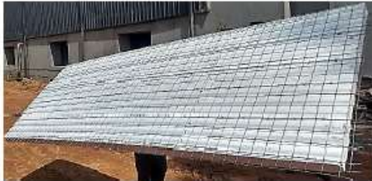
Fig. 1 Factory made EPS core panel and welded wire mesh reinforcement
