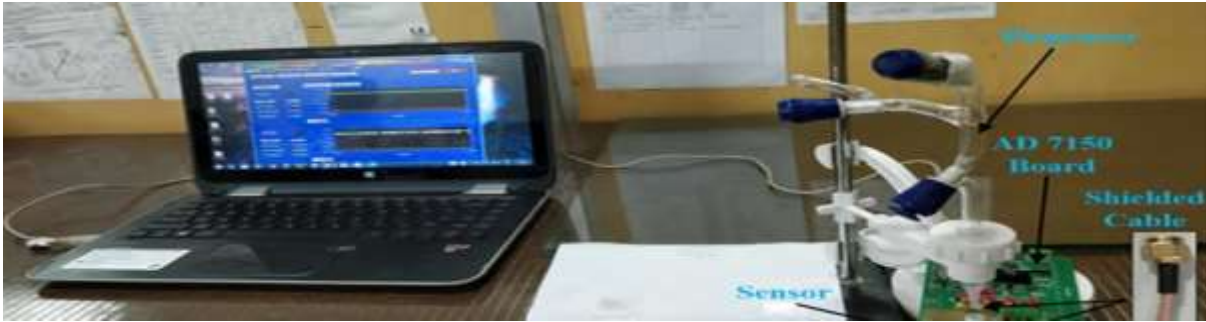
Cross-capacitive sensor experimental set up for micro droplet detection, DRDO project 2017-2020
