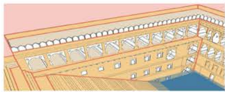
Diagram of a baoli with steps, a tank/basin, and well, positioned over the underground water aquifer
