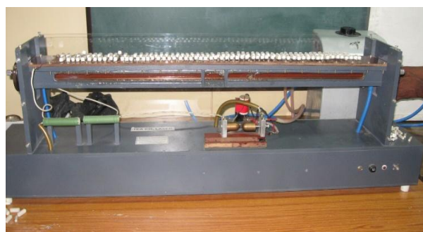
Figure 2. A Photograph of fabricated TEA CO 2 Laser
