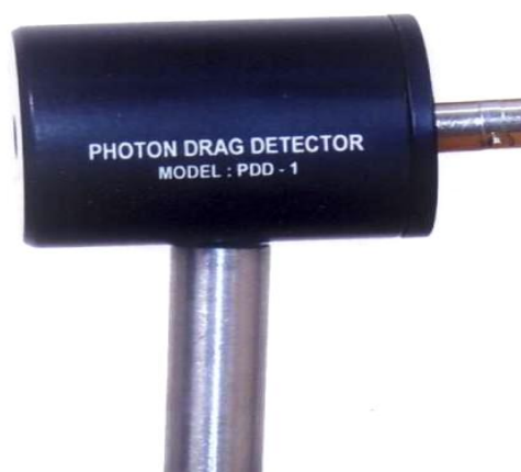
Figure: 1.A photograph of the fabricated Photon Drag Detector (Type A)
