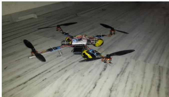
Smart Quadcopter is a next generation autonomous drone with image processing and tracking abilities. It incorporates a stabilized and flexible flight program which is made compatible with controls on android phone and laptops.
