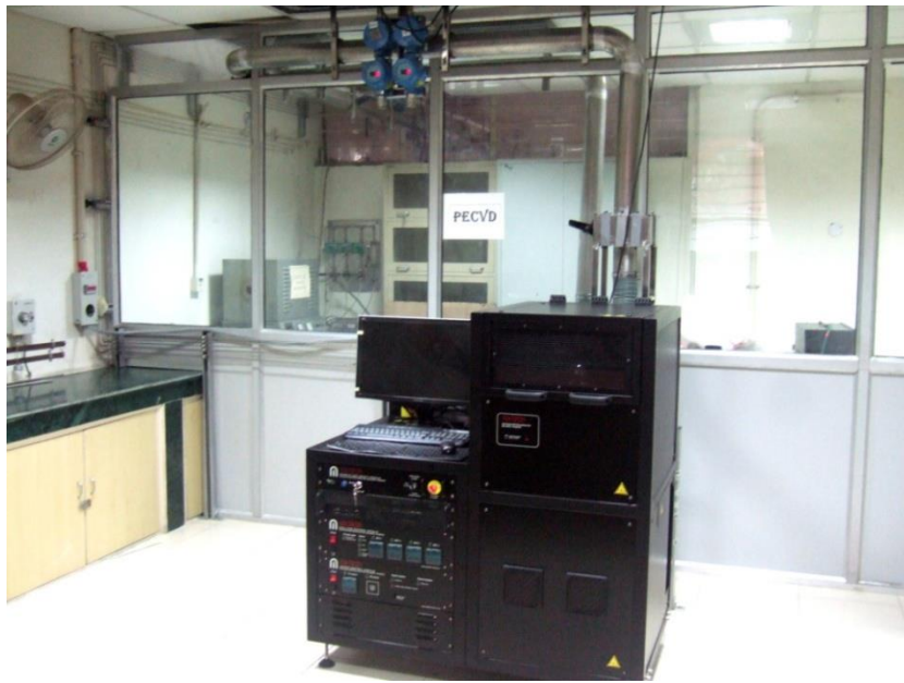
PECVD CNT Growth System with Enclosure Exhaust, JMI
