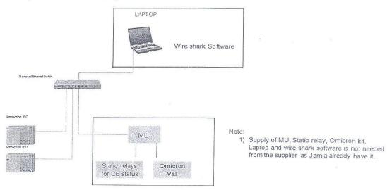
All the equipments supplied should support the type of Merging Unit and Omicron Kit available in Jamia Lab:-
